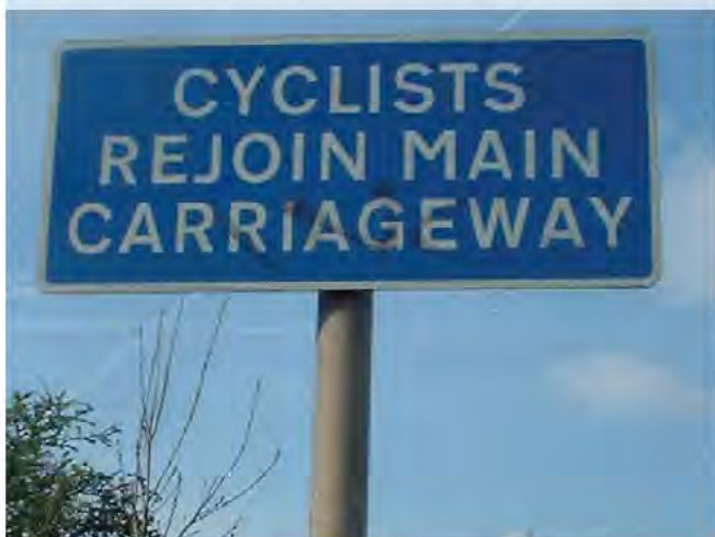
Figure 13.1: A positive instruction should be used where a sign is necessary to indicate the end of a route.
