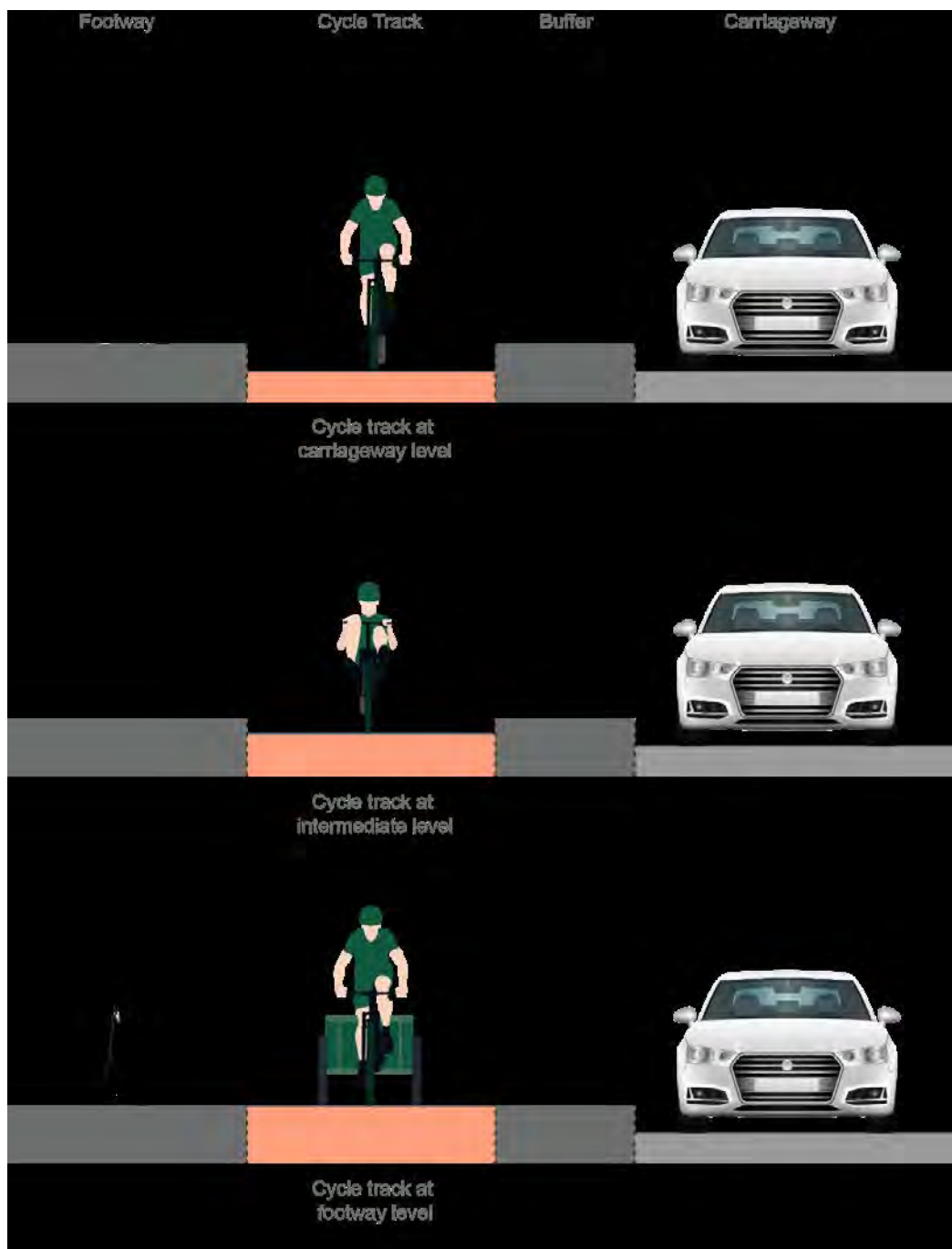
Figure 6.3: Cycle tracks with full kerb separation from carriageway
